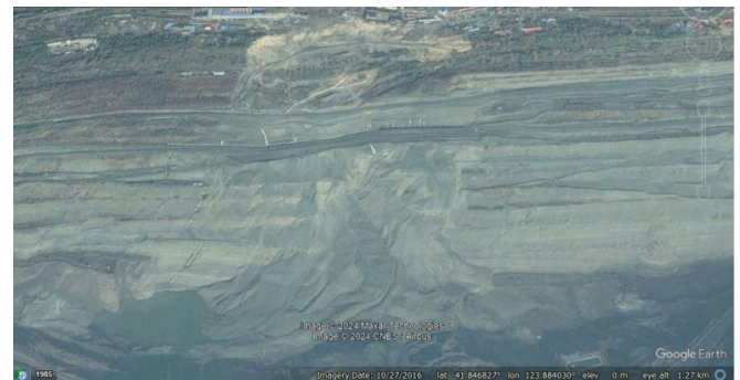
Google Earth image from October 2016 showing the failure at Fushun West OPM.
