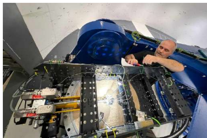
Markus Iten, a centrifuge technician, makes the final preparations before testing a model of a monopile supporting an offshore wind turbine. (Image: Ioannis Anastasopoulos / ETH Zürich)
